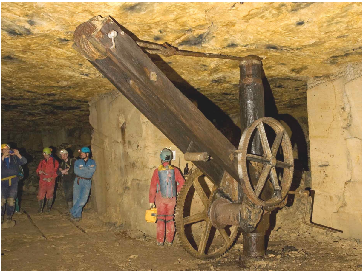
Wooden Crane, Box Stone Mine, Wiltshire.
