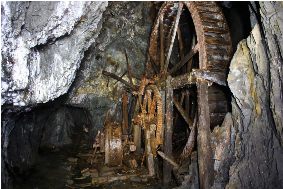
The underground waterwheel in the main drainage level. Photo P Sandbach
