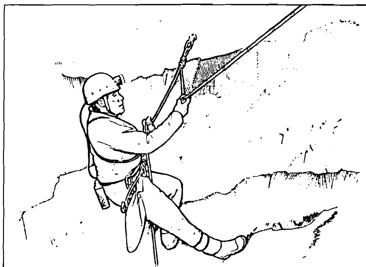
Starting the descent. When starting an abseil, check that everything is OK before unclipping the cow's tail and starting descent
