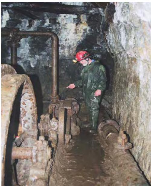
The winding drum is to the left in the foreground and JB is pointing to the crossheads on the engine.
