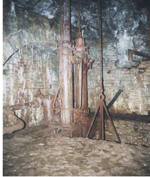
The above photo shows the two pump cylinders beside the top of the shaft.
