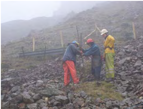
Probing the surface in order to determine the depth to the roof of the adit.
