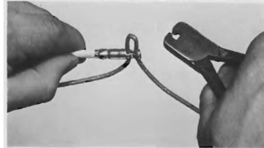
Fig. 26 Plastic Igniter Cord connected to safety fuse
