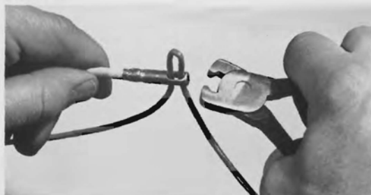
Fig. 24 Loop of igniter cord placed through aperture in 'beanhole' connector
