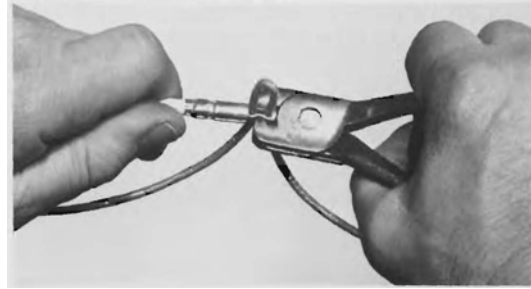
Fig. 26 Plastic Igniter Cord connected to safety fuse
