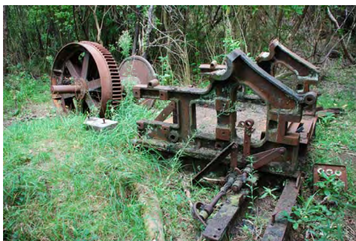
Winch base and winding drum, Puponga Coal Mine.
