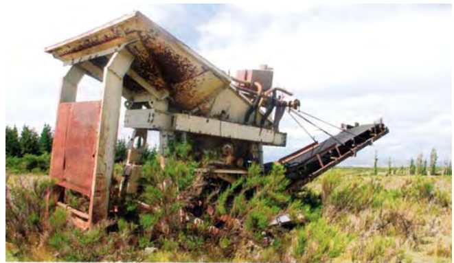
Abandoned portable gold extraction rig, at Tinkers (now Matakanui). Gravel fed through graded screens to fibre mats.
