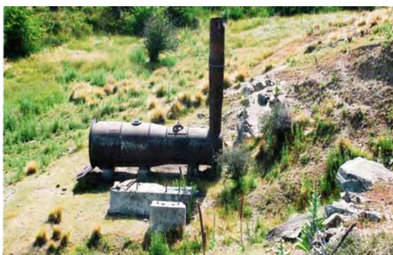
Golden Progress Mine battery. Viewed from the tramway. Note the two oil drums on the chimney for increased 'pull'!
