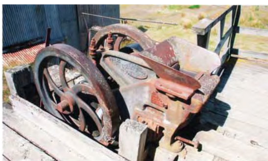
The ore was delivered by a tramway to a hopper which fed a Dodge stone breaker, the ore then passed into the battery to the stamps.
