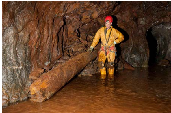
John Cameron stands beside what is assumed to be the remains of a rag and chain pump.
