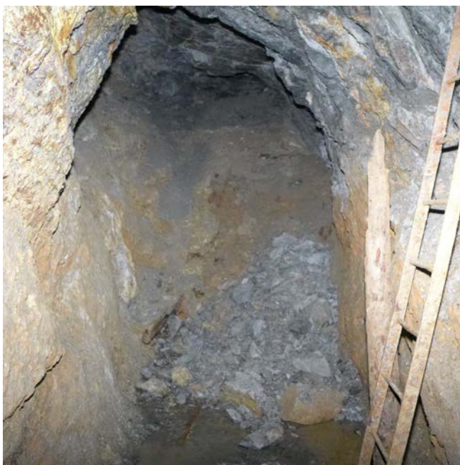
Fall as of the 30 th June prior to steel being installed
