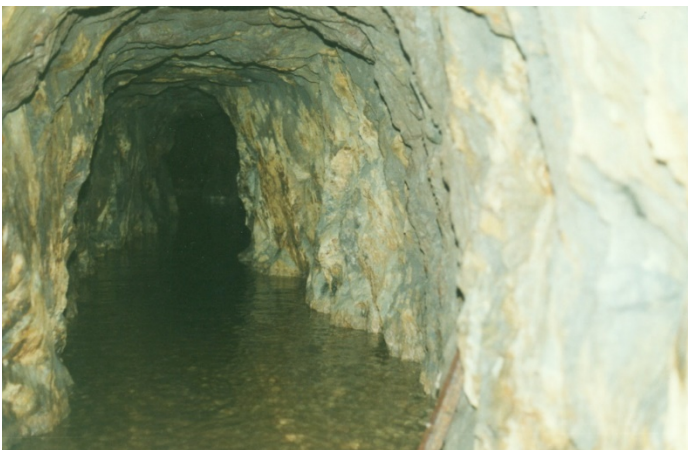
Crosscut from the Old vein to the East- West vein- Note the outline of the rails in the water
