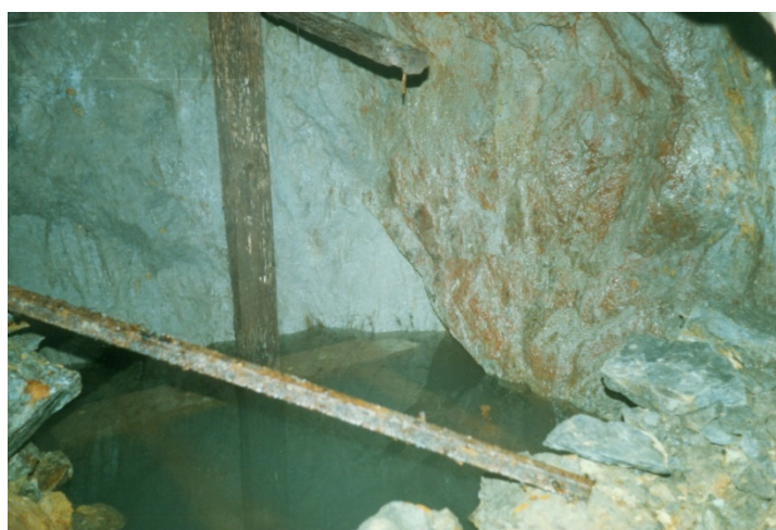
Flooded sump with remains of a jackroll on the Old vein
