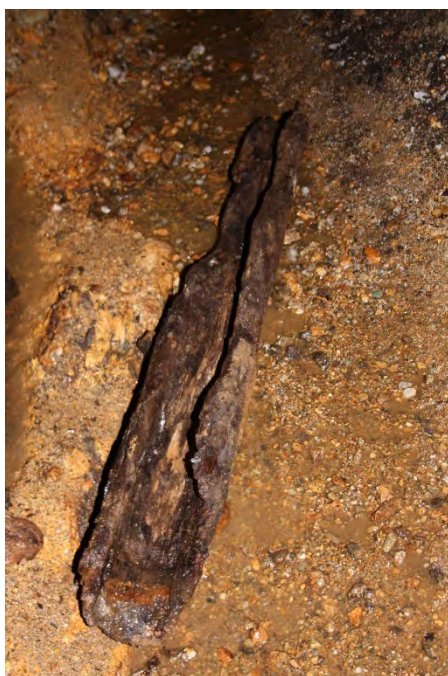
Left. Possible wooden pipe from a rag and chain pump
