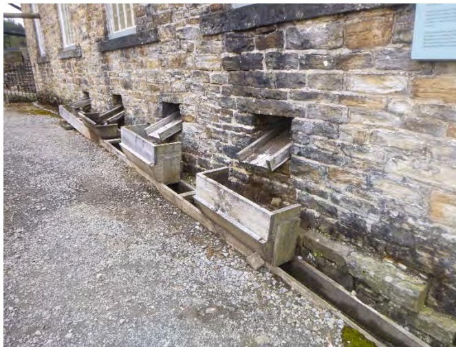
Launder carrying the waste from the jigs to the next process
