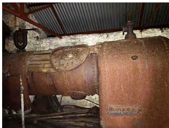
The steam plant, possibly taken from a traction engine. Photos M B Oddie.
