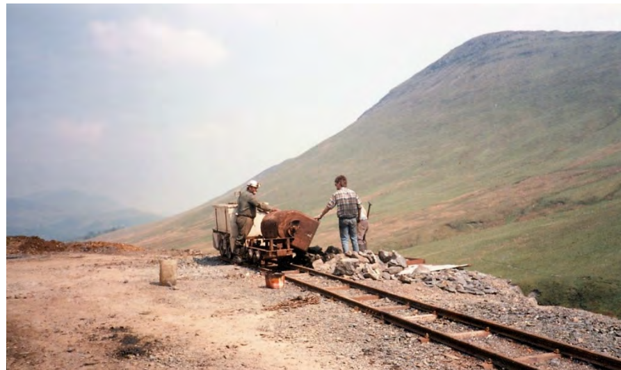
Lyndsay Greenbank, Neil Barnes and Ronnie Calvin tipping the ore into the grizzly.
