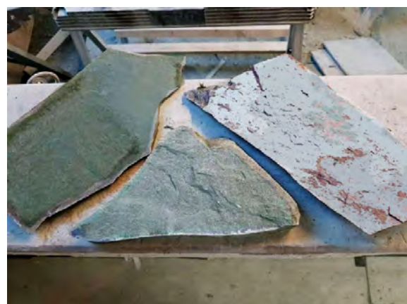
Left; Samples of slate brought down from Dale Head into the Honister workshop Right: Samples of slate freshly split and treated. The colour of the split surfaces clearly shown that the left hand sample (collected from B in the satellite image) is olive-green and therefore from the Kimberley slate band, centre sample (collected from C) is pale green and from the 'Honister' slate band and the right hand sample (collected from E) has a blue / grey tinge and is therefore from the Quay Foot slate band.
