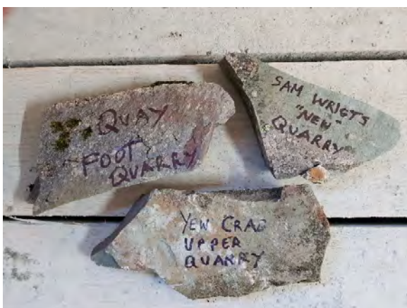
Left; Samples of slate brought down from Dale Head into the Honister workshop Right: Samples of slate freshly split and treated. The colour of the split surfaces clearly shown that the left hand sample (collected from B in the satellite image) is olive-green and therefore from the Kimberley slate band, centre sample (collected from C) is pale green and from the 'Honister' slate band and the right hand sample (collected from E) has a blue / grey tinge and is therefore from the Quay Foot slate band.
