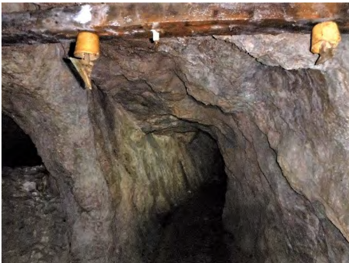
Two of the conductors back in place on an original timber.
