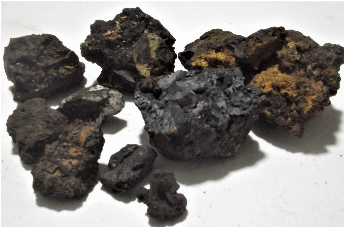
Examples of Iron rich Breccia with traces of Manganese, Goethite in centre.
