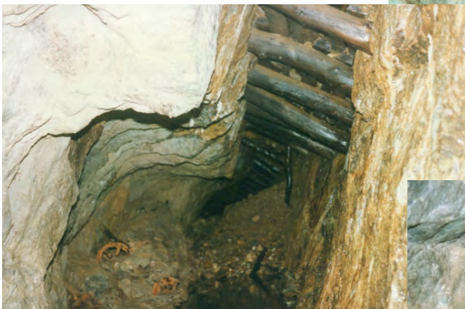
A rope was tied off around the original rail at No 2 shaft which gave access to the 75-fathom level, which had some superb timbering to support the stopes
