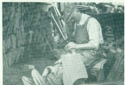
A reaver splits the slate to the correct thickness, and then the slate passes to the dressing floor.
