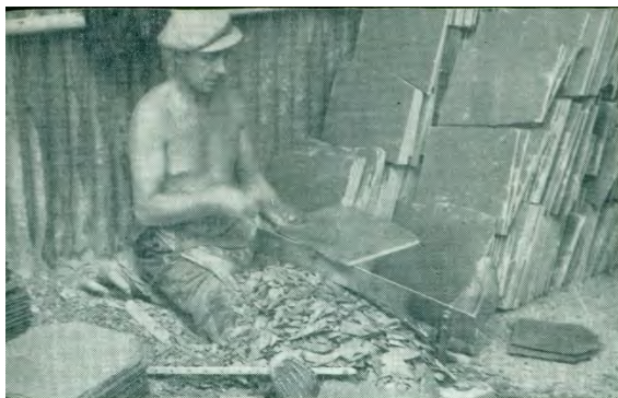
A dresser trims the slates to their final shapes. A stack of finished slates can be seen on the left.
