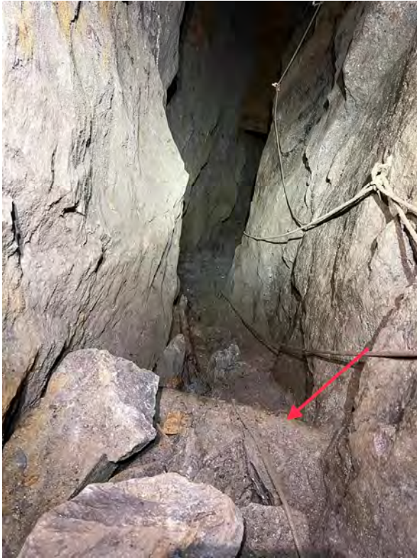
Arrow pointing at a stemple part covered in deads. The climbing chain is just behind me.
